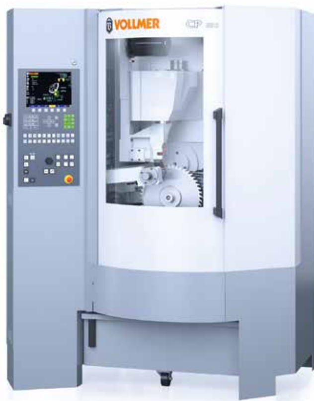
CP650: Sharpening machine for carbide tipped circular saws 硬质合金圆锯片刀磨机床
